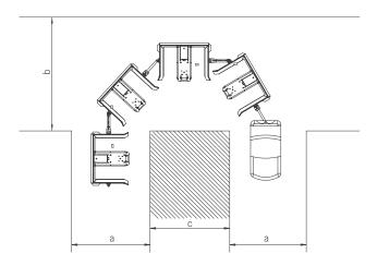
a = aisle widthb = aisle widthc = distance between the aisles
