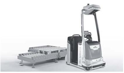
The LTX 50 iGo systems combine automated travel with automated load handling
