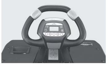
Unique STILL Easy Drive steering wheel for optimised driver control and operation of all functions without changing grip  $^{\rm 2}$
