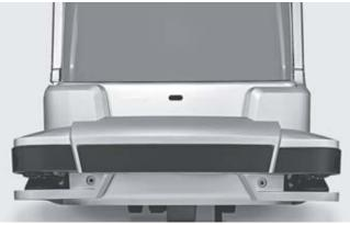
$360\,^{\circ}$  personal protection provided by integrated safety laser scanners in the LTX 50 iGo systems
