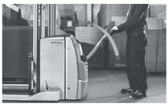
Safety as standard: depending on tiller angle, speed is automatically adapted to the distance between the operator and the truck (OptiSpeed)  $^{\rm 1,\,2}$
